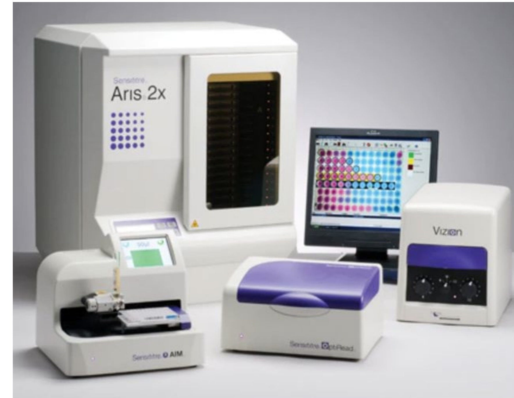
Figure 2: Complete Sensititre™ system includes ARIS™ 2x, Vizion™, AIM™ (Automated Inoculation Delivery System), Optiread™ (Automated Fluorometric Plate Reading System), and computer with SWIN™ software.
